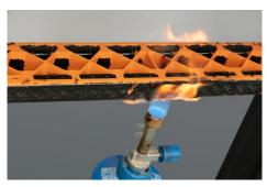
LANXESS' own fire test on a model carrier: The black carrier profile is made of one of the new Tepex grades, the rib structure of an orange, likewise halogen-free flame-retardant polyamide 6 Durethan. The flames do not spread, but extinguish when the burner is removed – regardless of whether the carrier is flamed over the surface or at the edges.
