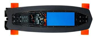
The trough-shaped deck houses all the electric and electronic functions, including the battery, except for the motors, which are mounted on the back of the skateboard.
